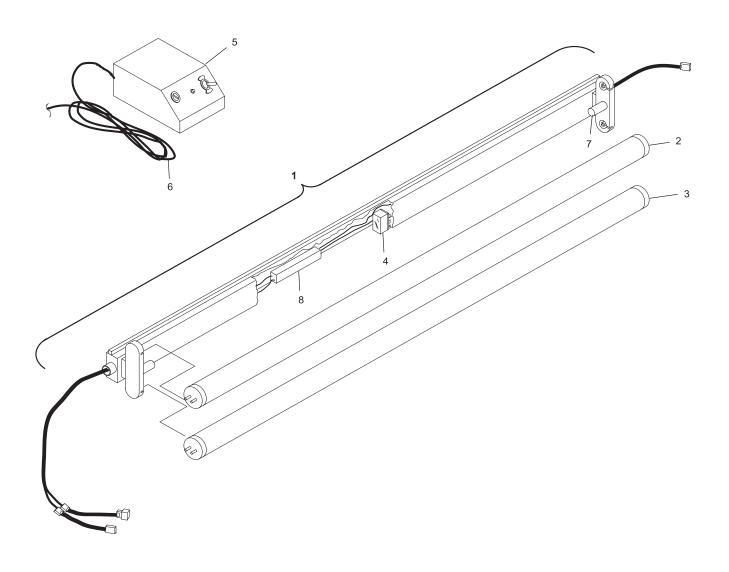
Dual Pin Lamp System (Machine Series 443 and Above)
